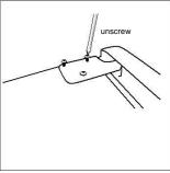
Remove the pin with a screwdriver and flip the hinge bracket.
