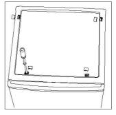
5. Unscrew top hinge and then remove upper door and place it on a soft pad to avoid scratch.
