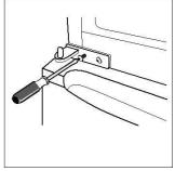
10. Place the upper door back on. Ensure the door is aligned horizontally and vertically so that the seal are closed on all sides before finally tightening the top hinge. Then inert the hinge and screw it to the top of the unit.
