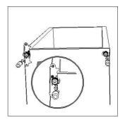
□ Make the middle hinge reverse the direction180° C, then transfer it to the left property position. Make the middle hinge pin in the upper hole of the lower door, then tight the bolts.
