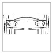
$\hfill\square$  Unscrew bottom hinge. Then remove the adjustable feet from both side.
