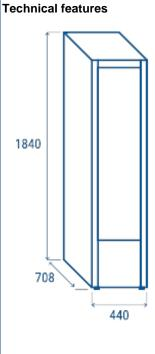
300 Lt. Upright slim cooler • White coated steel for internal and external side Roll-bond evaporator system with fan assisted cooling Automatic compressor cycle defrost Foaming Agent Cyclopentane (43mm per side) Mechanical thermostat Analog thermometer Air conveyed through a inner large fan Removable Gasket White adjustable shelves: 4 Pcs + 1 Pcs Bottom Self closing door Painted aluminium door frame with
