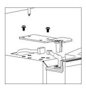
6. Lift the door and place it on a soft pad. Then remove another door as same process.
